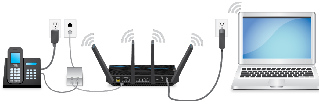
Figure 8. Modem router cabling for DSL service
