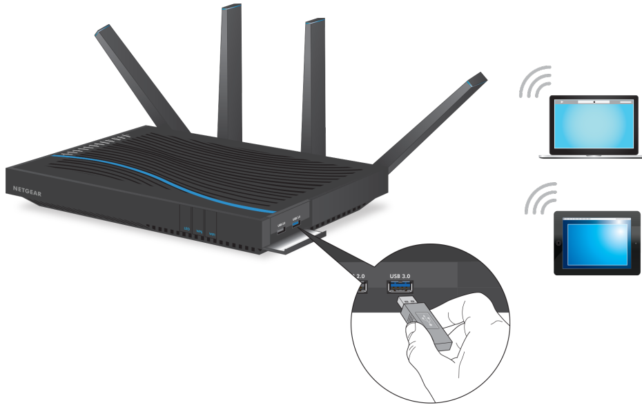
Figure 4. A USB 3.0 port and a USB 2.0 port are located on the right
