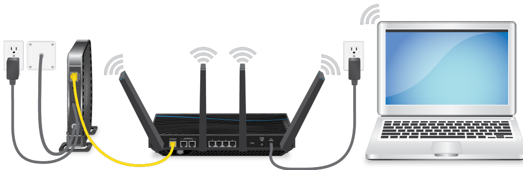
Figure 9. Modem router cabling for cable service
