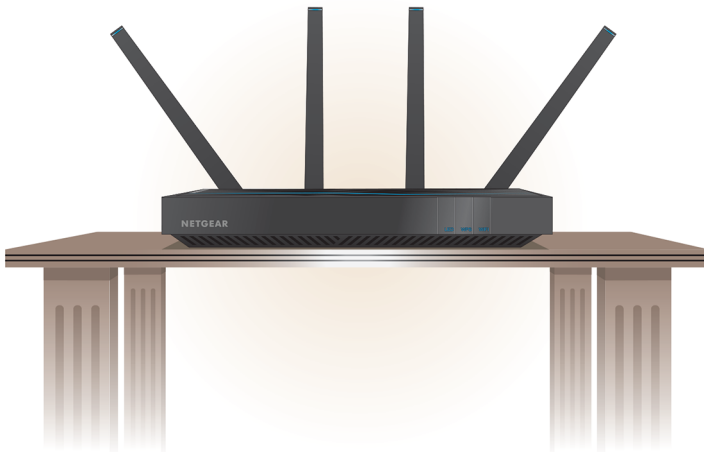
Figure 7. Two antennas in the center positioned vertically, the other antennas at a 45-degree outward angle
