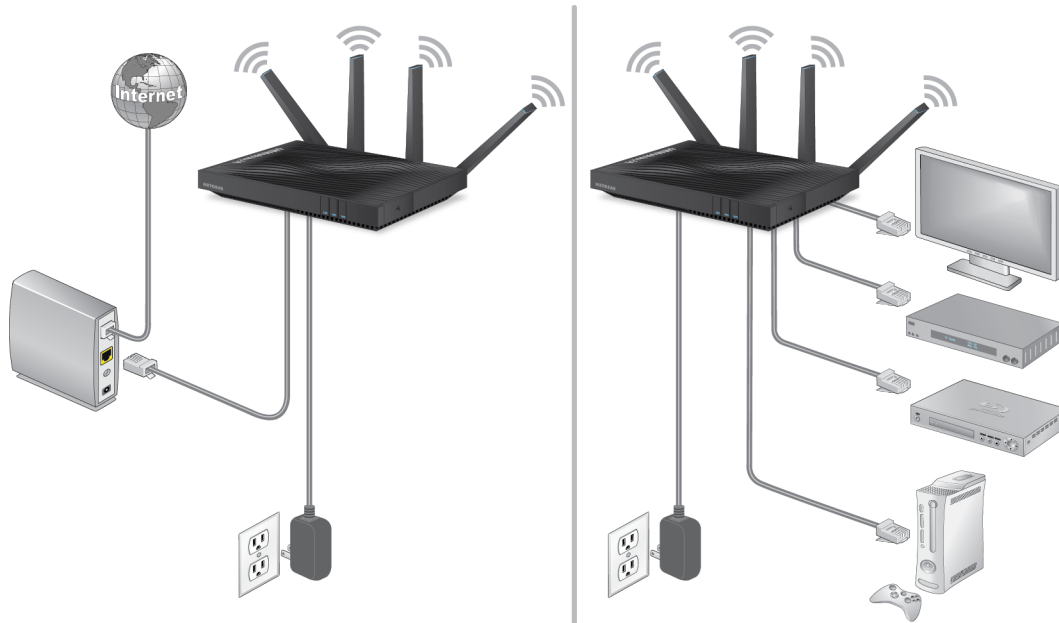
Figure 12. Router in bridge mode
