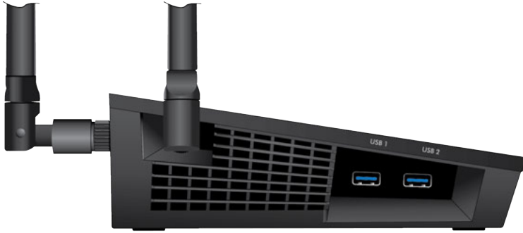
Figure 11. Two 3.0 USB ports are located on the side of the modem router
