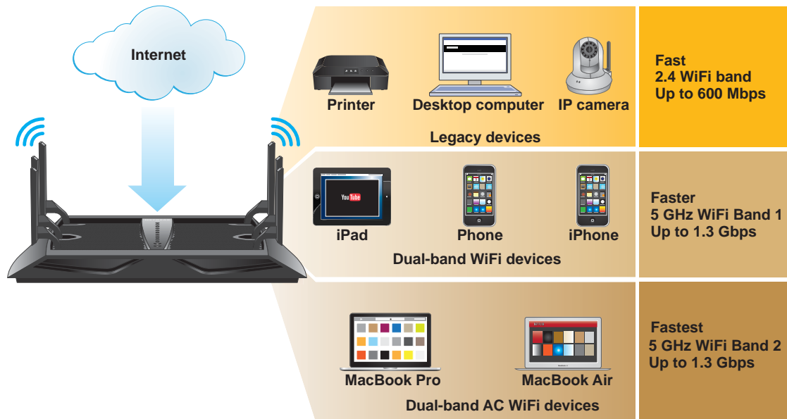
Figure 9. Load balancing in a tri-band WiFi network
