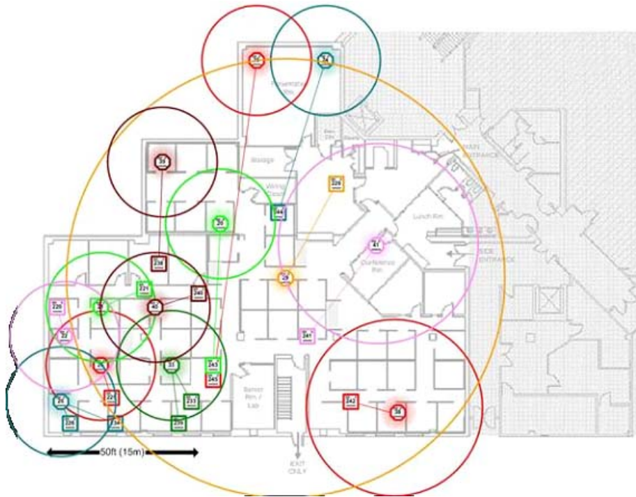
Figure 5-4: AutoCell View wireless network
