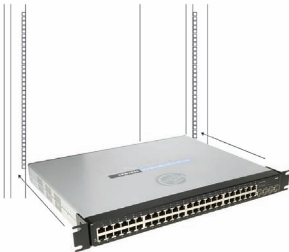
Mount the Switch in the Rack
