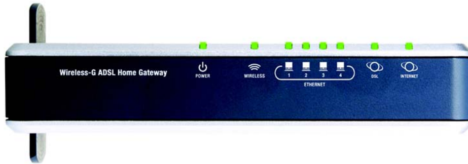
Figure 3-2: LEDs on Side Panel
