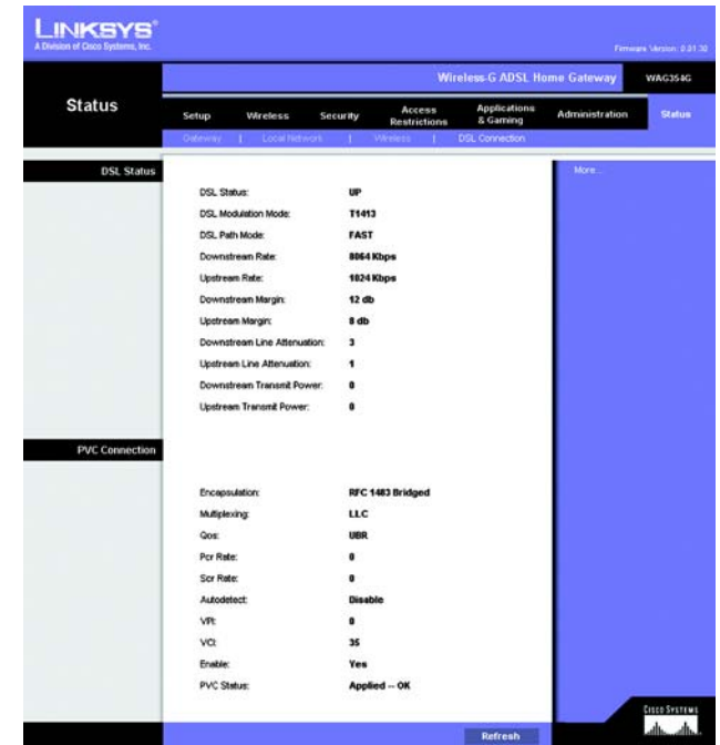
Figure 5-47 : DSL Connection (Connexion DSL)
