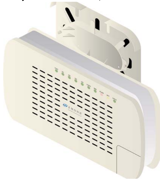
Figure 3: The unit may also be wall mounted, with or without a fiber tray
