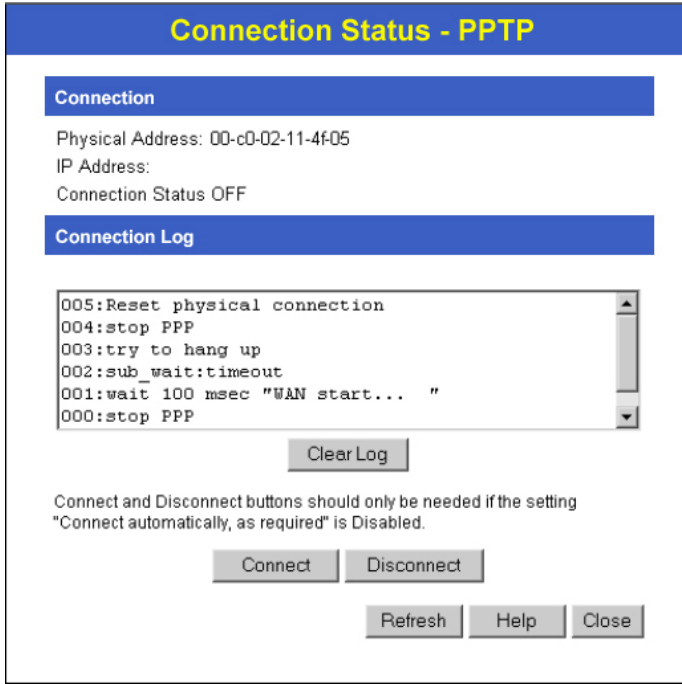
Figure 23: PPTP Status Screen
