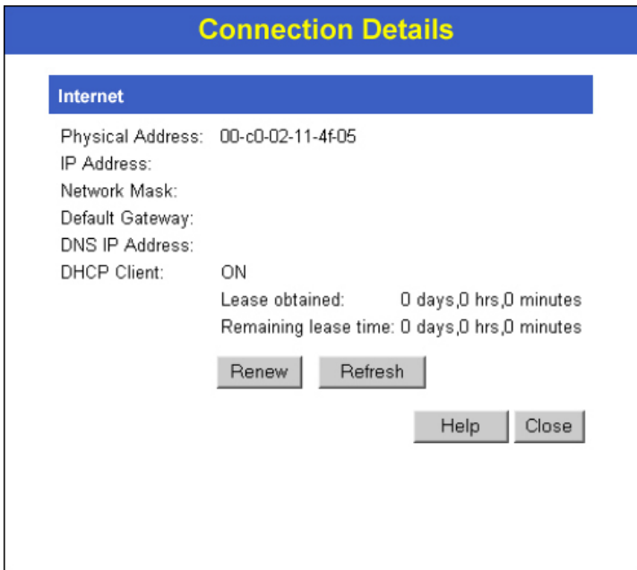
Figure 26: Connection Details - Fixed/Dynamic IP Address
