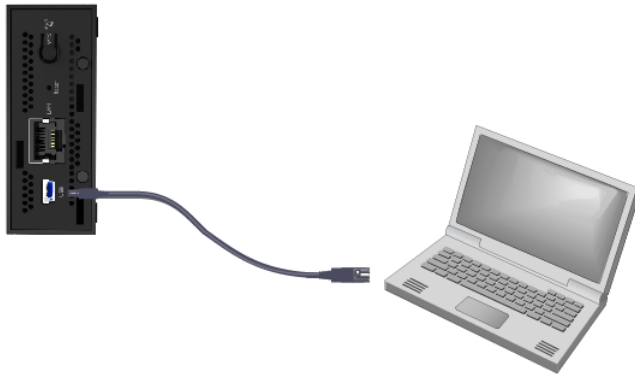
Figure 2. Connecting the WNCE3001 to a laptop
