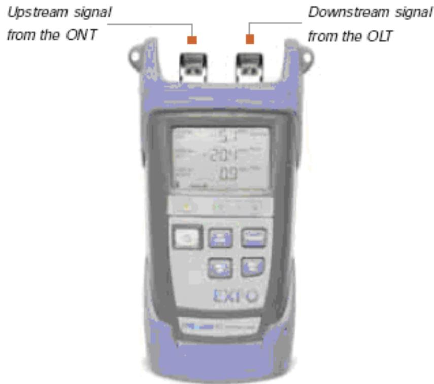
As shown in **Figure 5-2**, the PPM-350B optical power meter is different from common optical power meters. Specifically, the PPM-350B has a downstream input optical port and an upstream
