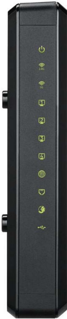
Figure 4 LEDs on the VMG
