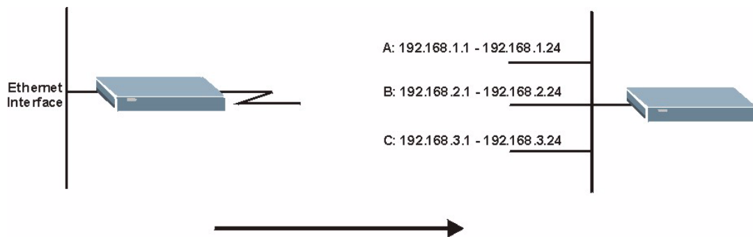
Figure 38 Physical Network & Partitioned Logical Networks
