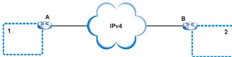
Figure 182 Configured Tunnel Example
