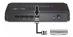
5. Connect one end of a network cable to one of your router LAN ports (1-4). Connect the other end of the network cable to the computer Ethernet port (also called network port).
