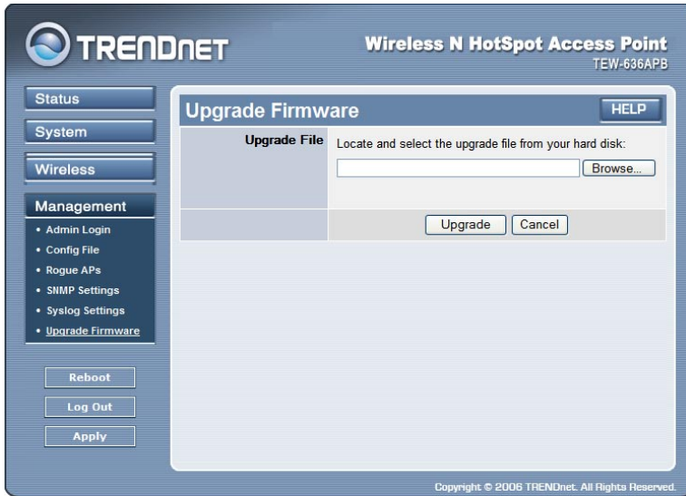
Figure 61: Firmware Upgrade Screen
