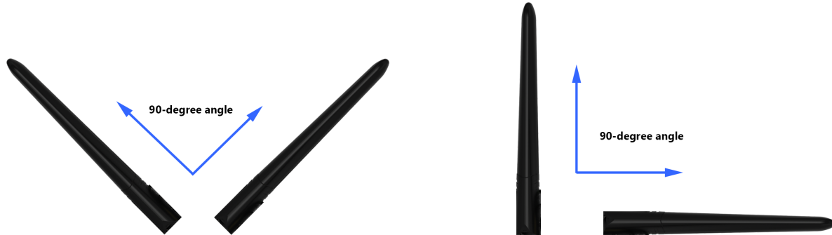
Figure 3. Examples of recommended antenna positions
