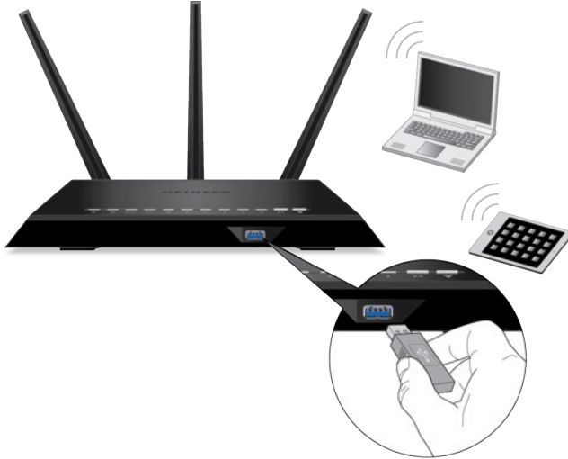
Figure 10. One 3.0 USB port is located on the front panel of the router
