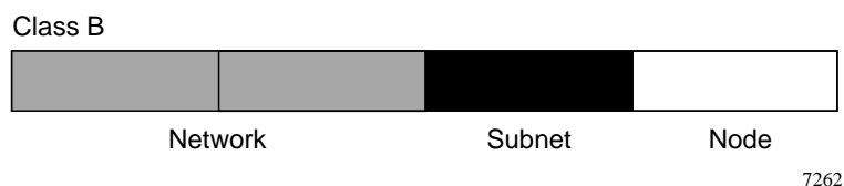
Figure 6-2: Example of Subnetting a Class B Address
