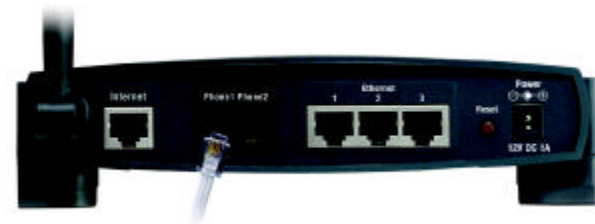
Figure 4-3: Connect a Telephone
