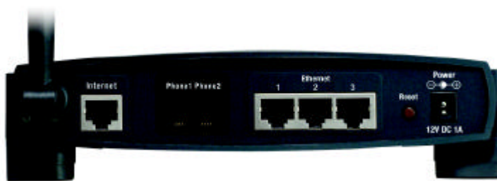
Figure 3-1: The Broadband Router's Back Panel
