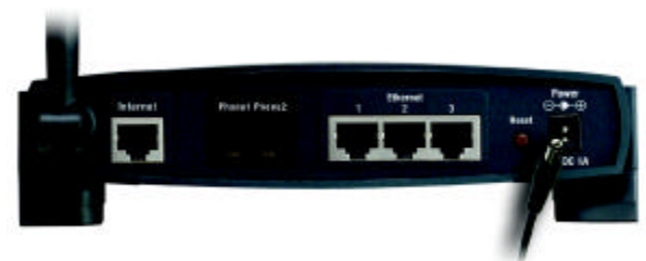
Figure 4-5: Connect the Power
