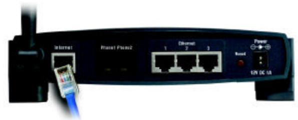
Figure 4-4: Connect the Cable/DSL Modem
