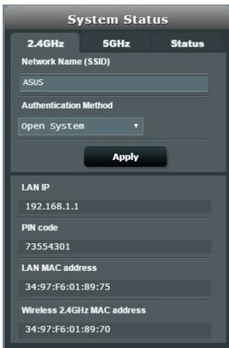
The screenshot shows the 'System Status' screen for the 2.4GHz band. It features three tabs: '2.4GHz', '5GHz', and 'Status', with '2.4GHz' selected. The 'Network Name (SSID)' field contains 'ASUS'. The 'Authentication Method' dropdown menu is set to 'Open System'. Below these fields is an 'Apply' button. Further down, the LAN IP is '192.168.1.1', the PIN code is '73554301', the LAN MAC address is '34:97:F6:01:89:75', and the Wireless 2.4GHz MAC address is '34:97:F6:01:89:70'.
