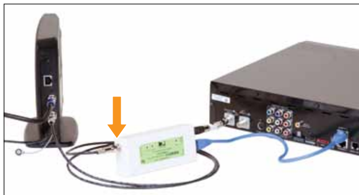
Connect Enclosed Coaxial Cable to "Towards LNB" on the Connected Home Adapter
