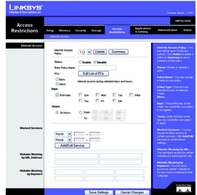
Figure 5-44: Access Restrictions Tab - Internet Access
