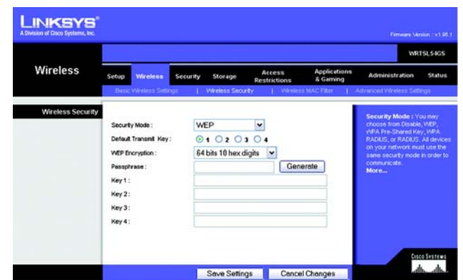
Figure 5-26: Wireless Tab - Wireless Security (WEP)
