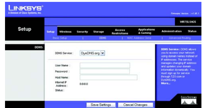
Figure 5-13: Setup Tab - DDNS (DynDNS.org)
