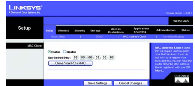
Figure 5-15: Setup Tab - MAC Address Clone
