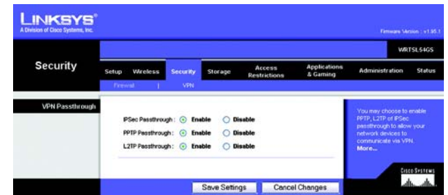
Figure 5-31: Security Tab - VPN Passthrough
