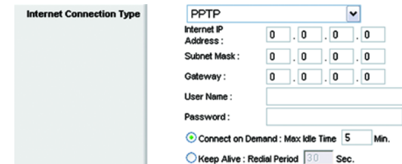
Figure 5-6: PPTP Connection Type
