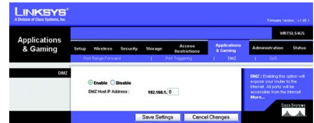
Figure 5-50: Applications and Gaming Tab - DMZ
