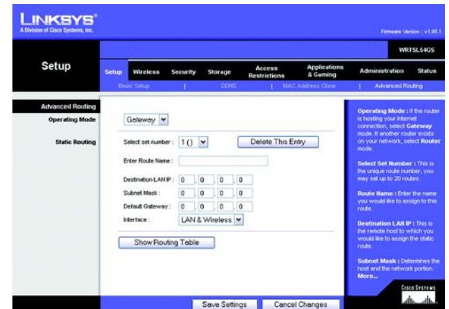
Figure 5-16: Setup Tab - Advanced Routing (Gateway)
