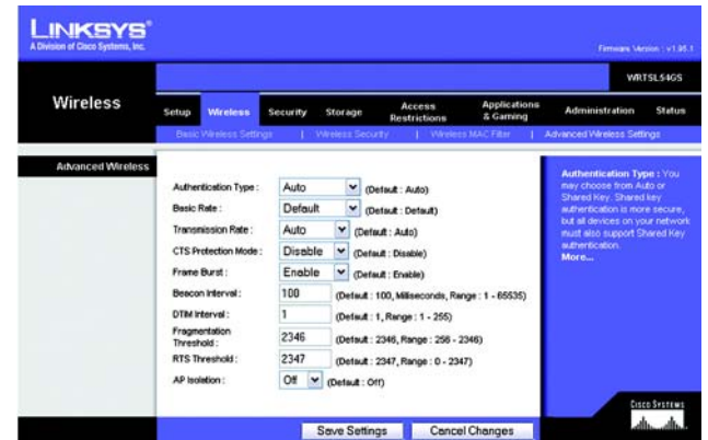
Figure 5-29: Wireless Tab - Advanced Wireless Settings
