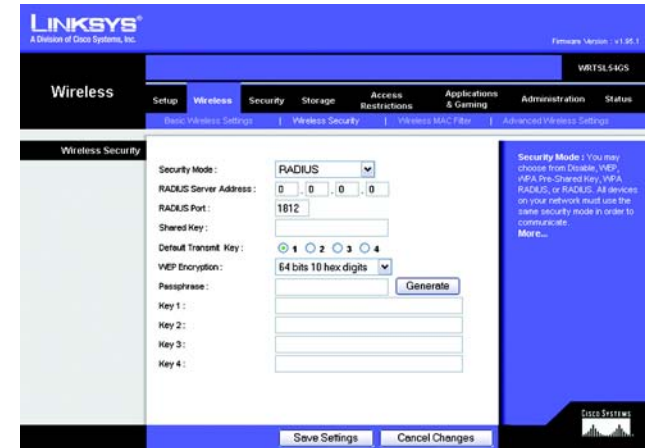
Figure 5-25: Wireless Tab - Wireless Security (RADIUS)
