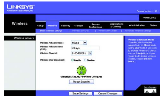
Figure 5-19: Wireless Tab - Basic Wireless Settings
