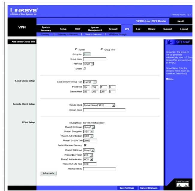
Figure 6-45: Client to Gateway
