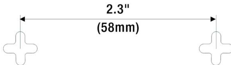
Figure D-1: Wall-Mounting the Router
