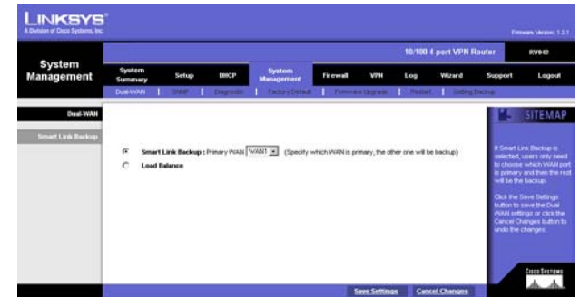
Figure 6-22: Dual-WAN Smart Link Backup
