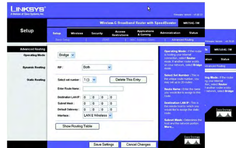
Figure 5-16: Setup Tab - Advanced Routing (Bridge)
