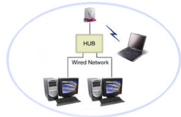
Figure 2. Extending a Wired Network
