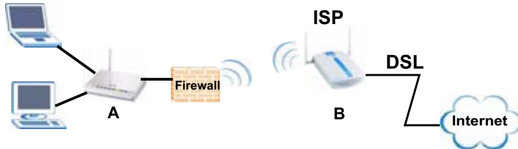
Figure 2 Using the P-320W v3 as a Wireless Client
