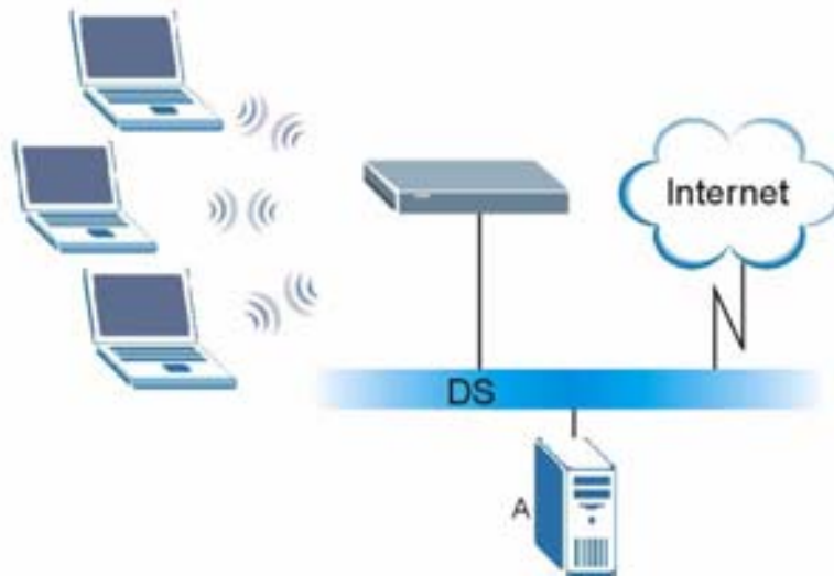
Figure 31 WPA with RADIUS Application Example
