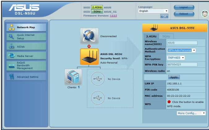
4. On the **Wireless name (SSID)** field, key in a unique name for your wireless network.
