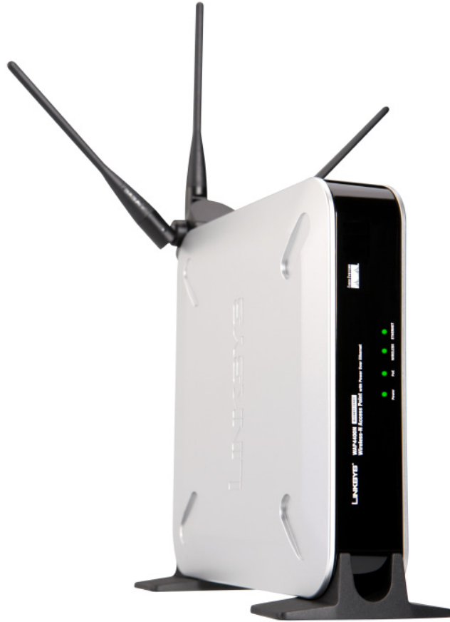
Figure 3-4: Standalone Position and its Antenna Setup
