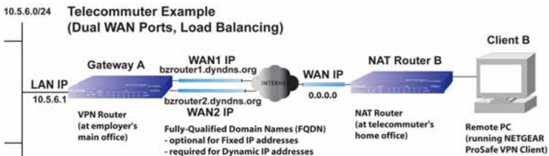
Figure 32. Telecommuter example in a dual WAN port configuration with NAT and load balancing
