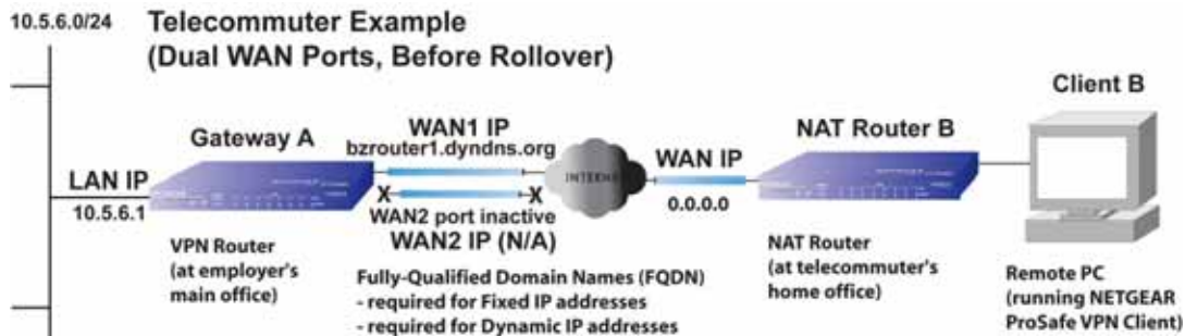
Figure 30. Telecommuter example in a dual WAN port configuration with NAT before auto-rollover
