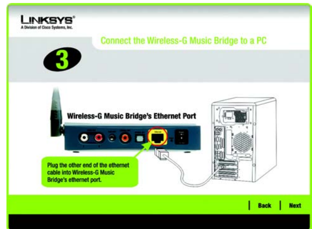
Figure 3-4: Connecting the PC to the Bridge
