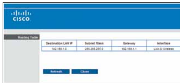
Advanced Routing > Routing Table
