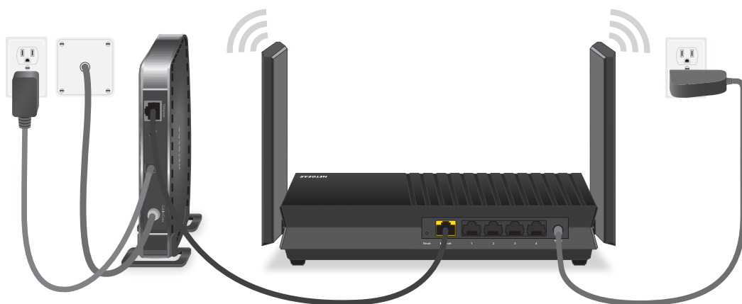
Figure 6. Cable your router
