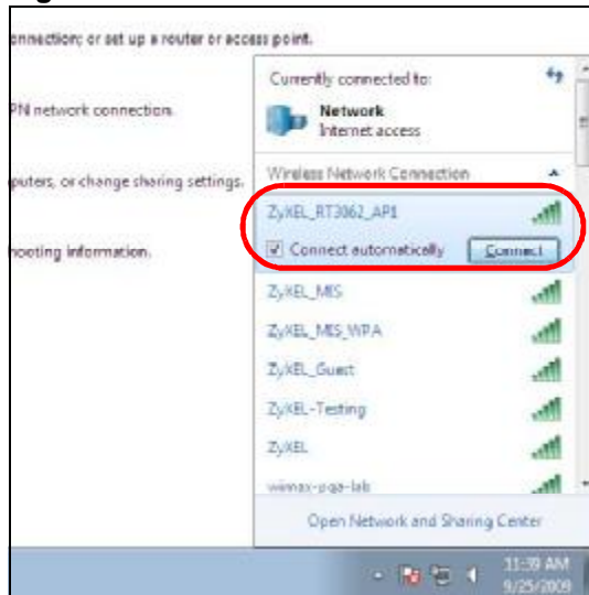
Figure 150 Windows 7: Connect to the Wireless Networks
