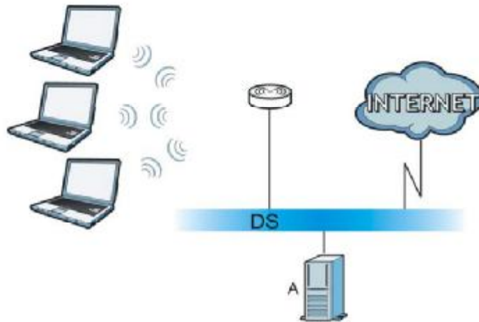
Figure 112 WPA(2) with RADIUS Application Example
