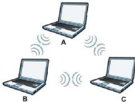
Figure 108 Peer-to-Peer Communication in an Ad-hoc Network
