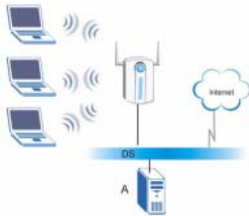
Figure 9 WPA with RADIUS Application Example
