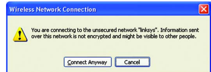
Figure B-5: No Wireless Security
